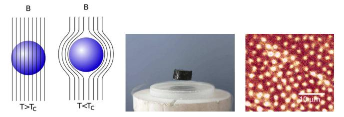
The Meißner effect (left) expels a magnetic field from a superconductor, leading to levitation in type-I superconductors (centre), and to Nielsen-Olesen flux tubes in type-II superconductors (right).
