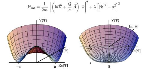
Ginzburg-Landau potential for the superconducting phase,  $\lambda > 0$  (left); for the normal phase,  $\lambda < 0$  (right).
