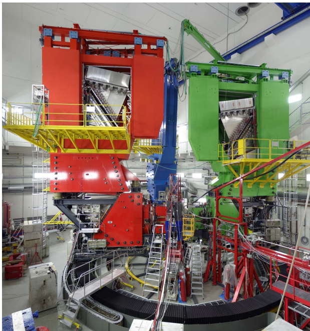
Fig. 5.4. Experimental set-up for the measurement of electron scattering off protons and nuclei at the electron accelerator MAMI-B (Mainzer Microtron). The maximum energy available is 820 MeV. The figure shows three magnetic spectrometers. They can be used individually to detect elastic scattering or in coincidence for a detailed study of inelastic channels. Spectrometer A is shown in cutaway view. The scattered electrons are analysed according to their momentum by two dipole magnets supplemented by a system of detectors made up of wire chambers and scintillation counters. The diameter of the rotating ring is approximately 12 m. (Courtesy of Arnd P. Liesenfeld (Mainz), who produced this picture) [PRSZR]
